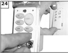
Remove cover by snapping off from top or bottom. Install 12V battery into wall remote. Duracell MN21/Eveready A23/GP 23A all 12V
